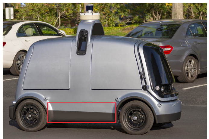
Image: Location of the traction battery (red rectangle)
